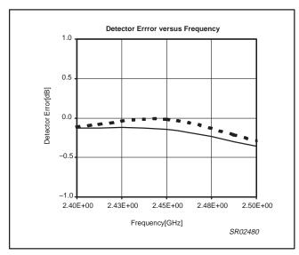
Figure 19. Detector error vs. frequency
